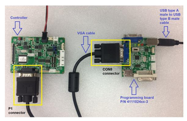
3. Insert 12V power source to PP2 connector and short JP6 / power on the DT-1920-VGA.
