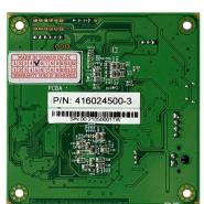
EPM-050 Driver Board: Designed specifically to support the E lnk 13.3" monochrome panels, the EPM-050 accepts bitmap images transferred over a USB connection. The images are then written to the panel immediately. The board has fast startup and ultra low standby power consumption of 0.01W (for 5V inpput).
