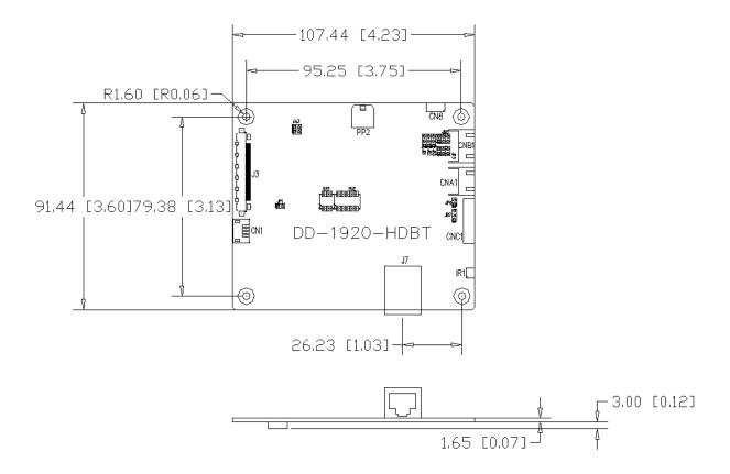
The maximum thickness of the controller is 13.95mm (measured from bottom of PCB to top of components, including any underside components & leads). We recommend clearances of:
