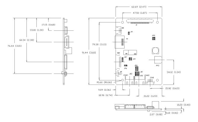
The maximum thickness of the controller is 13.95mm (measured from bottom of PCB to top of components, including any underside components & leads). We recommend clearances of:
