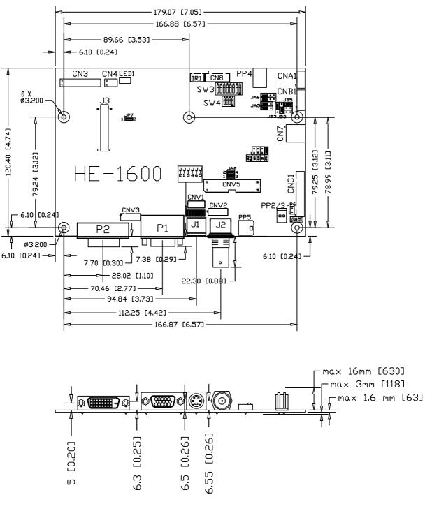
The maximum thickness of the controller is 20.6mm with or without video add-on board (measured from bottom of PCB to top of components, including any underside components & leads). We recommend clearances of:
