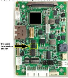
It provides three ways to read the on-board temperature value :
