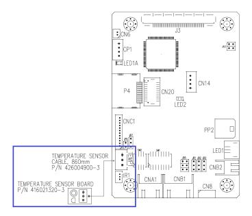
Read the external temperature sensor value via RS-232 command :
