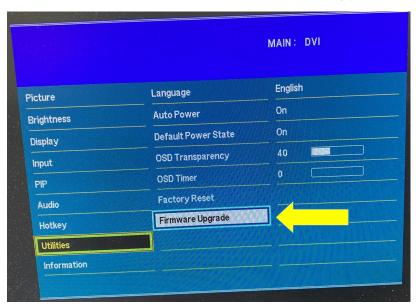
**Step 4 :** Press "+" on OSD switch mount to select 'Yes' for confirmation to perform the firmware upgrade process.
