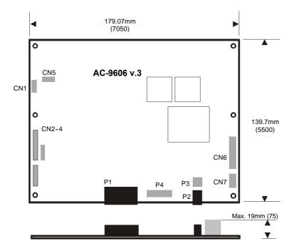
The maximum thickness of the controller is 19mm or 31mm with an inverter mounted on the controller (measured from bottom of PCB to top of components, including any underside components & leads). We recommend clearances of:
