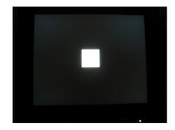
**Warning** - If the Auto Color Gain is executed without an appropriate image being displayed, then the process will set incorrect values and the display colors will be distorted. If this occurs, then it can either be corrected by performing the process correctly or if this is not possible then the Reset Color Gain function can be used. This function will reset the stored RGB values to a set of approximate values.
